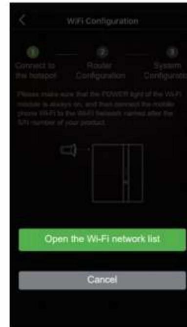
Step 3 If your phone is not connected to the system hotspot, open the WiFi network list. Find the hotspot with the product SN in the WiFi list, enter the password "12345678" and connect to it.
